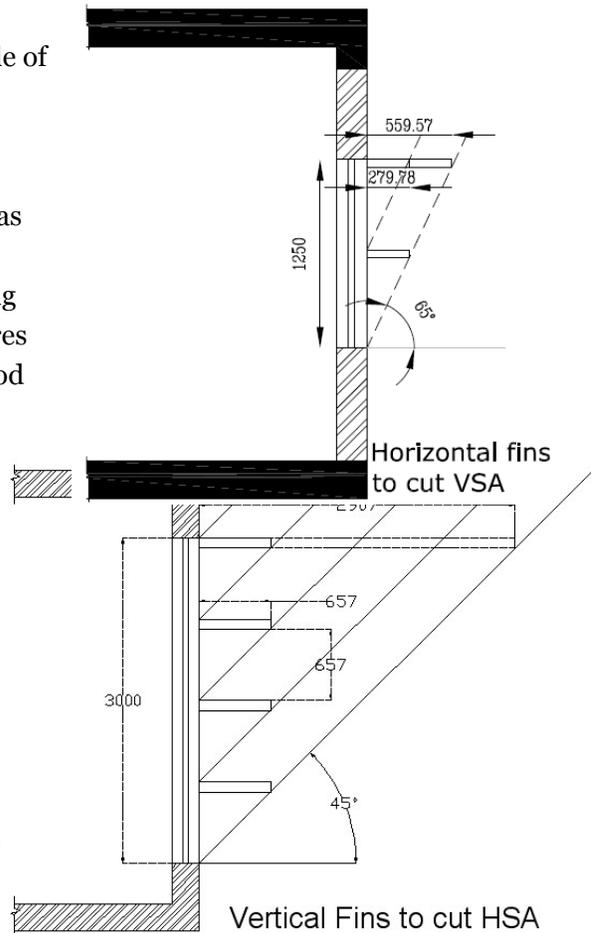
Design of shading device to cut the HSA
