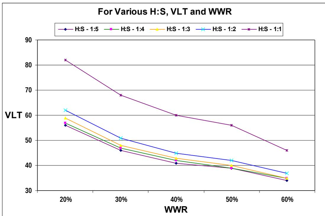
Example explaining the above graph – If two buildings are located such that the H:S is 1:2, then to achieve the adequate daylight in a space having 60% WWR one need to provide a glass of VLT around 37% or for the same H:S as 1:2 and for a glass of VLT around 45% the WWR around 40% will be required for adequate daylighting.
